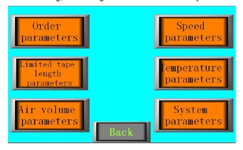
Limitted tape length paramters: To set the tapping length of the end tapping and then machine will auto cut the tape.
